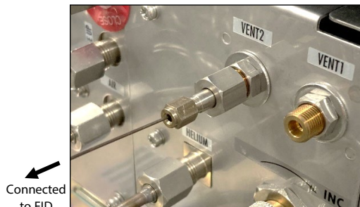
Fig. 4 BID Vent Connected to FID with Metal Column
