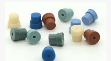
Septa are used to seal the injection port, allowing syringe to penetrate and introduce sample into the injection port without carrier gas leakage.
